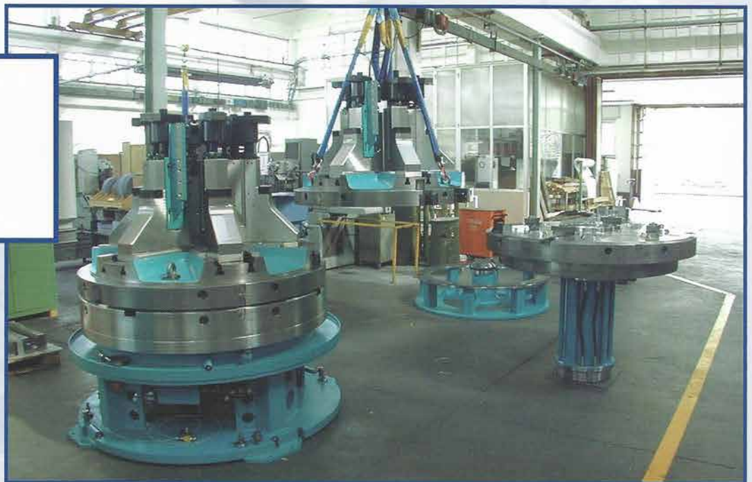
PALLETS EXCHANGER WITH PALLET TRANSFERRED BY CRANE
